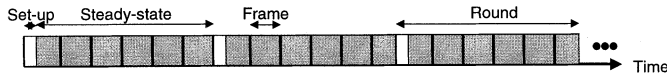
Fig. 1. Time line showing LEACH operation. Adaptive clusters are formed during the set-up phase and data transfers occur during the steady-state phase.
