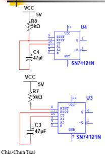
Q: 0V-5V-0V Pulse T=0.693RC=0.693\*5k\*47μ =162.855ms R=  $1.4k\Omega\sim40k\Omega$  C=0~1000μF
