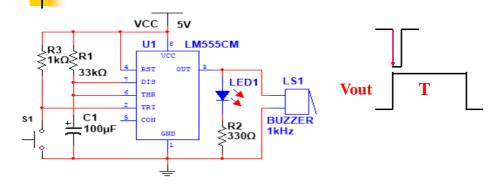
Push S1 once, LED1 & Buzzer are on for a time,
