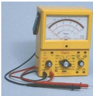
(b) Analog multimeter (VOM)
