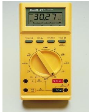
(a) Hand-held digital multimeter (DMM) (Reproduced with permission from the Fluke Corporation)
